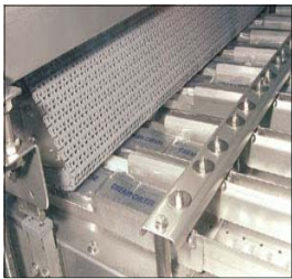
CUSTOM METERING BELTS Including Finned Belt for fragile products and O-head Mat Top for Pouch/Bars
