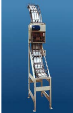
CUSTOM METERING BELTS Including Finned Belt for fragile products and O-head Mat Top for Pouch/Bars
