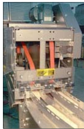
CUSTOM METERING BELTS Including Finned Belt for fragile products and O-head Mat Top for Pouch/Bars
